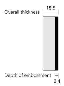
Besides the allowance of +/-0.3 mm of the total area thickness referring to the highest point there are minor differences in the thickness of the embossment - with a max. of 3.4 mm due to the natural design specifications
