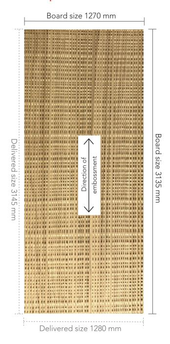
Besides the allowance of  $\pm$ 0.3 mm of the total area thickness referring to the highest point there are minor differences in the thickness of the embossment - with a max. of 1.2 mm due to the natural design specifications.
