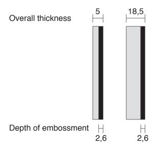
Besides the allowance of +/-0,5 mm of the total area thickness referring to the highest point there are minor differences in the thickness of the embossment - about 0,2 - 2,8 mm due to the natural design specifications.
