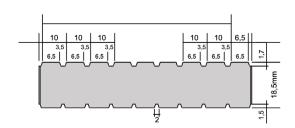
Besides the allowance of +/-0,5 mm of the total area thickness referring to the highest point there are minor differences in the thickness of the embossment - up to a maximum of 1,7 mm.
